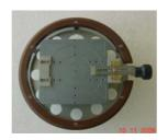
For components up to 4 x 4" Vacuum and mech. clamping
